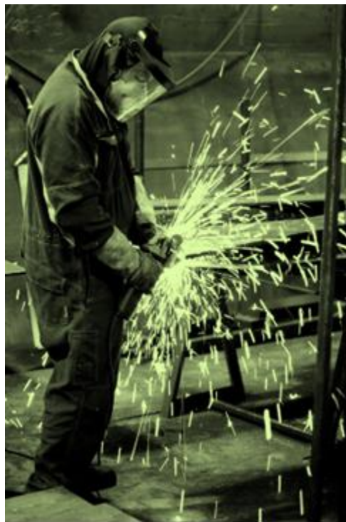
Figure 12 – Part finishing after welding
