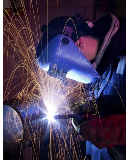
Figure 4 - Particle projection during GMAW welding
